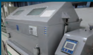
Salt fog test IEC 68-2-11
