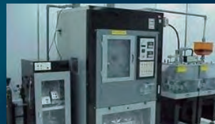
Gases corrosion IEC 60068-2-42/43
